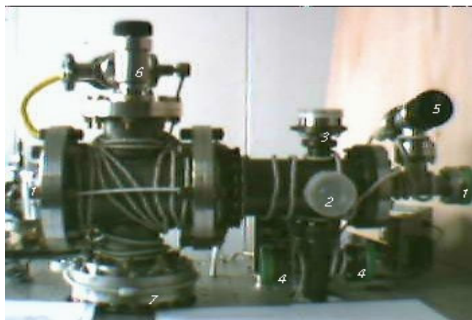
Fig2 INFLPR MOT: (1,2,3)-cooling optical windows; (4)-detection optical windows; (5)-thermal atoms source
